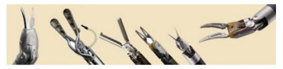
Figure 35: EndoWrist® instruments of da Vinci Surgical System
