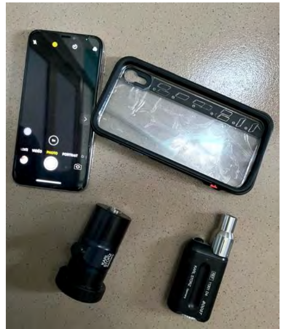
Figure 3 a: Simple solutions using a smartphone and adapter to the scope and a diode light source. (Photo courtesy Emmanuel Nzau Ngoma)
