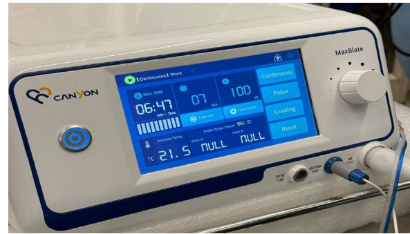
Figure 3: The Canyon KY 2000A MWA system. Note that the wattage is set at 100 Watts, the total time is at 7 minutes and the run time at the time of taking this picture is 6 minutes and 47 seconds. Probe temperature as recorded is 21.5 degrees Celsius.
